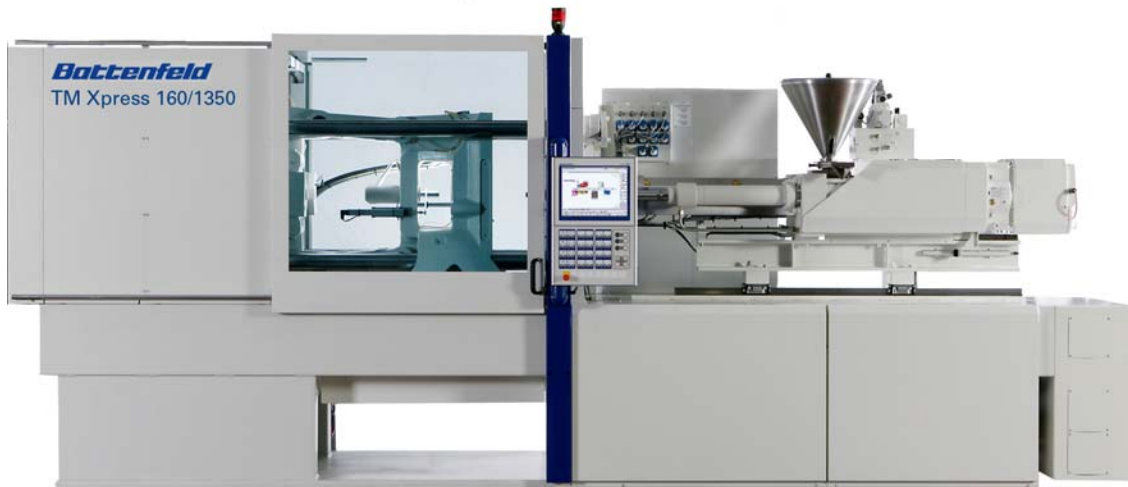
Fig. 1: The production of a PP butter tub with an IML application is demonstrated on a TM Xpress 160/1350
