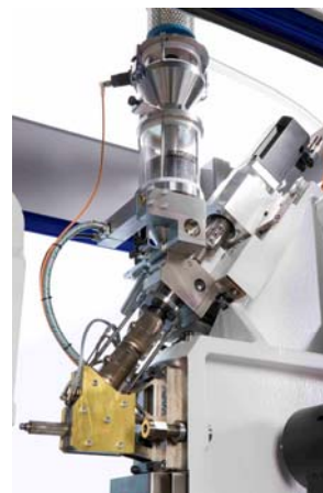
Fig. 7: Injection unit of the MicroPower
