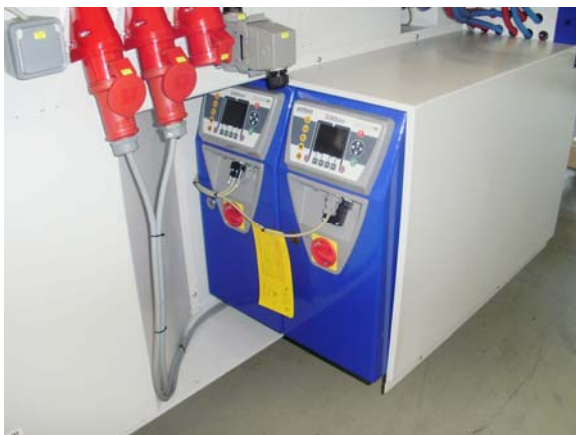
Fig 3: Integration of the TEMPRO plus C tempering device in the machine frame
