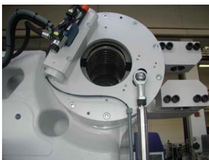
Fig. 4: Locking system “Quicklock”
