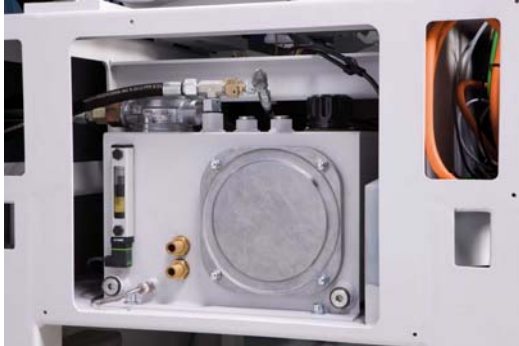
Fig. 2: Servo-hydraulics for peripheral movements
