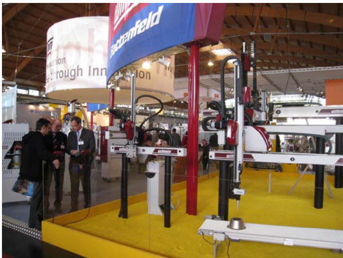
Fig. 2: The efficient Wittmann R8 robot control system permits the implementation of the interactive real time functions SmartRemoval , EcoMode , SoftTorque and PartTrack . This allows minimal removal times and economical, safe movements of all axes.
