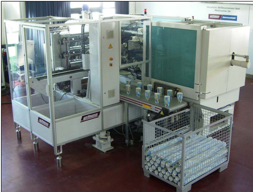
Fig. 1: 750 ml containers are manufactured on a TM Xpress 270/1350 with an IML system.
