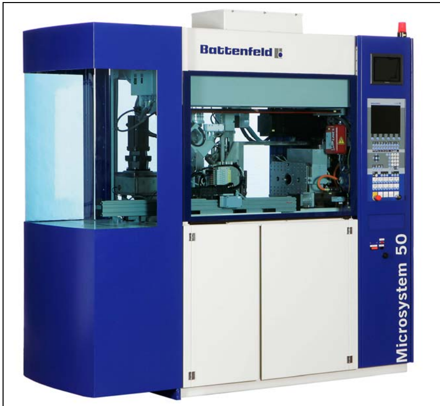
Fig. 5: The Microsystem 50 enables high precision system solutions for micro injection molding.
