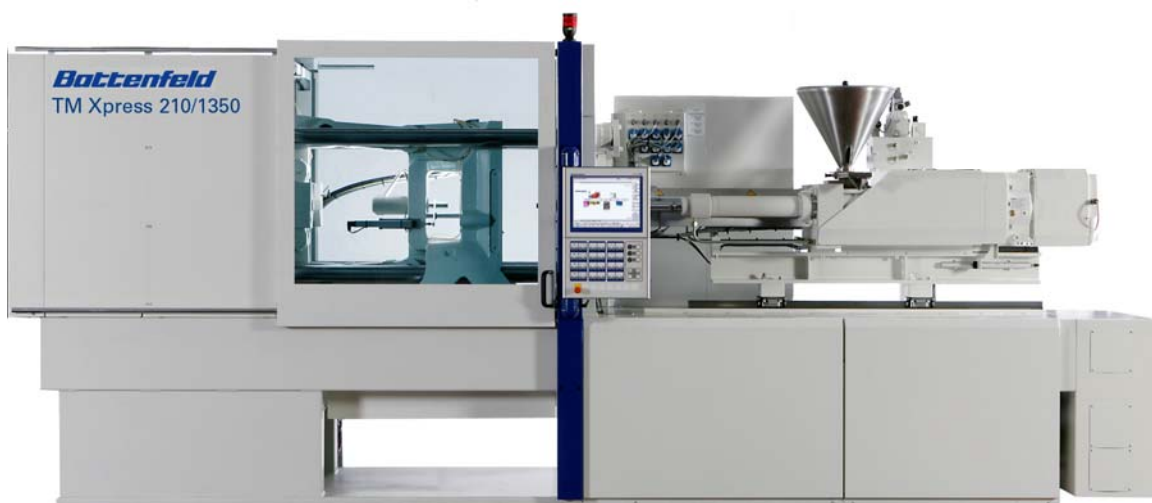
Fig. 1: During Brasilplast, the powerful high-speed model TM Xpress 210/1350 manufactures lids for PP ice-cream cups.
