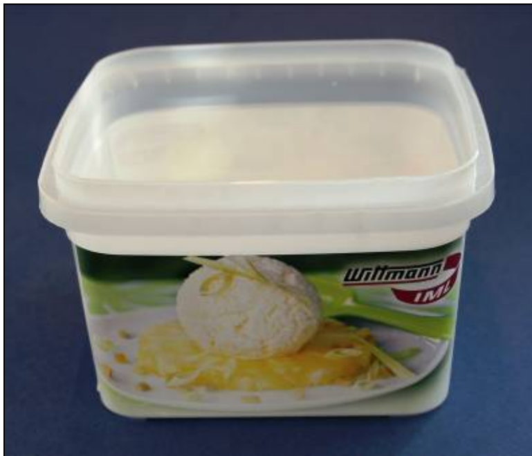
Fig 2: IML cups made of PP, manufactured on a TM Xpress 270/1350
