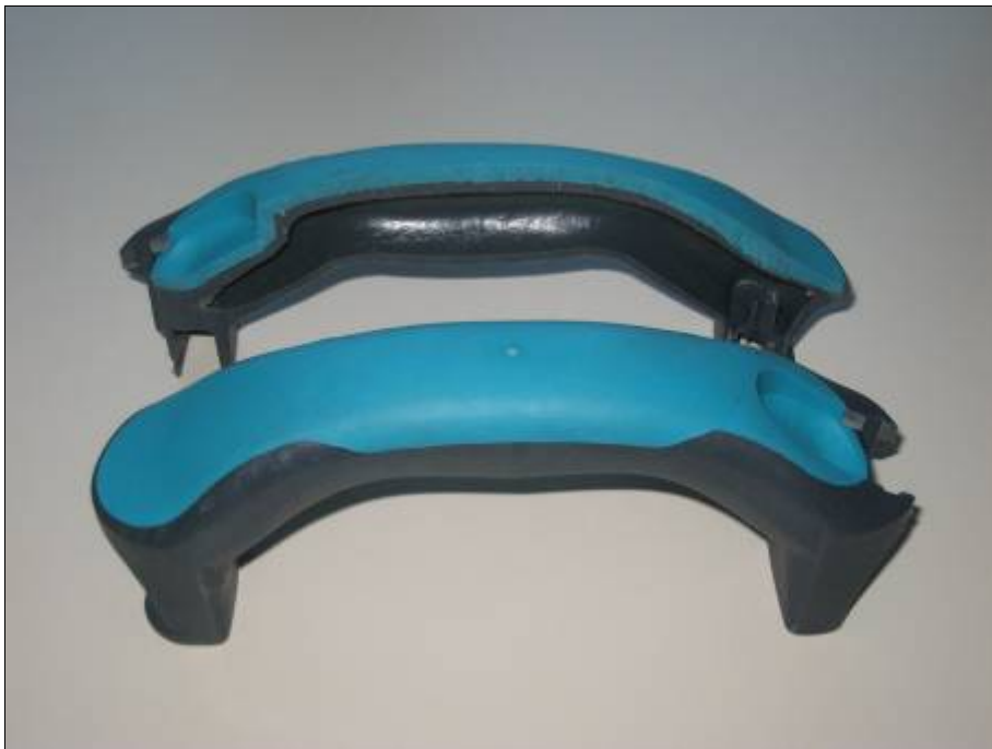
Fig. 5: 2-K handle with a cavity
