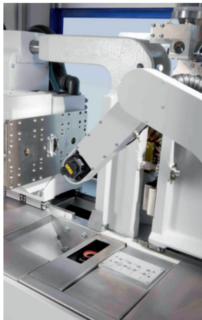
Fig. 5. Standard modules, such as robots, camera, stacking units and special automation solutions, can personalize the workspace. The neat machine internals offer an ideal basis for cleanroom applications
