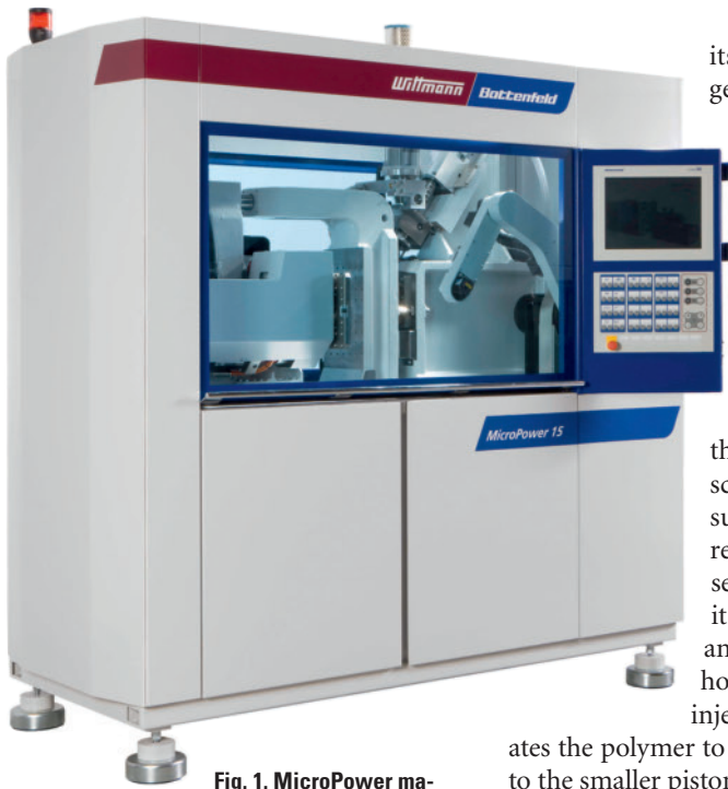
Fig. 1. MicroPower machines are available in two sizes; the 150 kN clamping force version is
